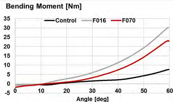
Figure 3. Results of the FAST forefoot bending stiffness measurement system of the different footwear conditions.
